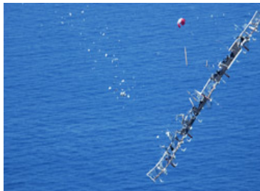
NASA Helios Mishap 1 . Left: Pitching oscillations and dihedral angles beyond design limit (aeroelastic response). Right: Structural disintegration resulting from critical loads
