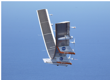
NASA Helios Mishap 1 . Left: Pitching oscillations and dihedral angles beyond design limit (aeroelastic response). Right: Structural disintegration resulting from critical loads
